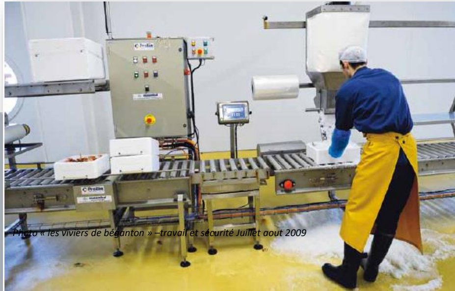
Direct and full automatic ice delivery into boxes
